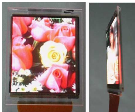
Fig. 5. Picture for the 2.2 inch AMOLED. (This figure is available in color, see the on-line version.)
